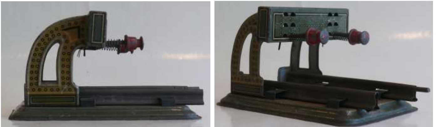
The last one is only marked Made in Germany. It allows to set different gauges and also different buffer widths and heights.
