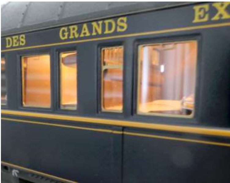
As mentioned this type sleeping car is named Z since it was the first with non-straight, i.e. Z like walls between the compartments to gain extra room for the wash basin, which is modelled correctly as can be seen in the picture above.
