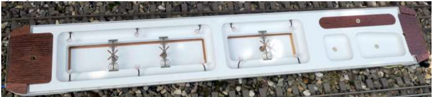
The roof is easily removed to show the detailed interior. The inside of the roof is also nicely detailed, including fans and lights
