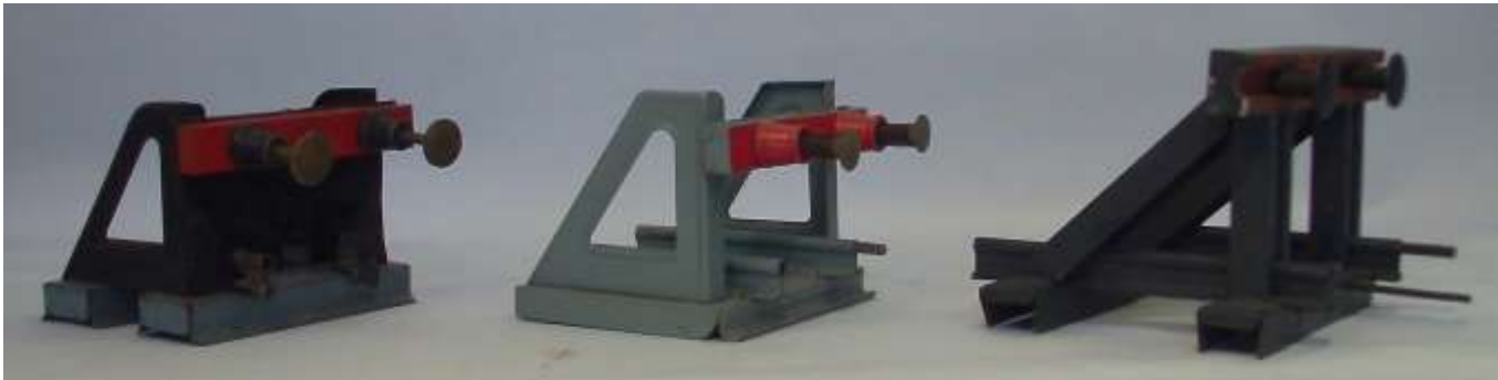
The next three are a bit messy; the left is marked Germany and looks as though it can bear no shock. The middle is a Bing buffer. The right is applicable for multiple gauges; also the buffer width and height can be adjusted on a rickety way.
