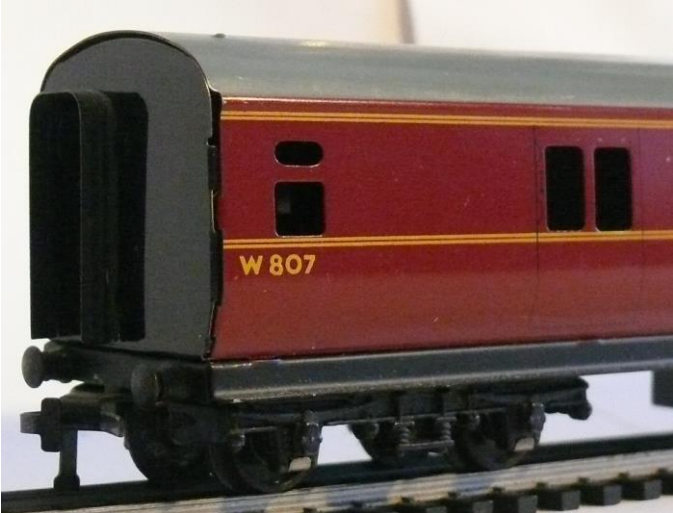
Note the prototypical correct asymmetric position of the corridor connection. This was to make sure that postal van corridors were only available between postal vans and the general public in a train could not enter a postal van.
