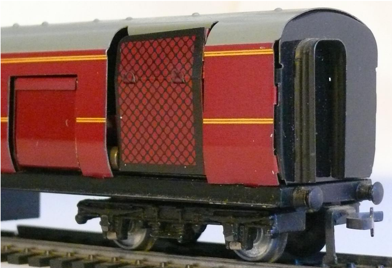
Note the prototypical correct asymmetric position of the corridor connection. This was to make sure that postal van corridors were only available between postal vans and the general public in a train could not enter a postal van.
