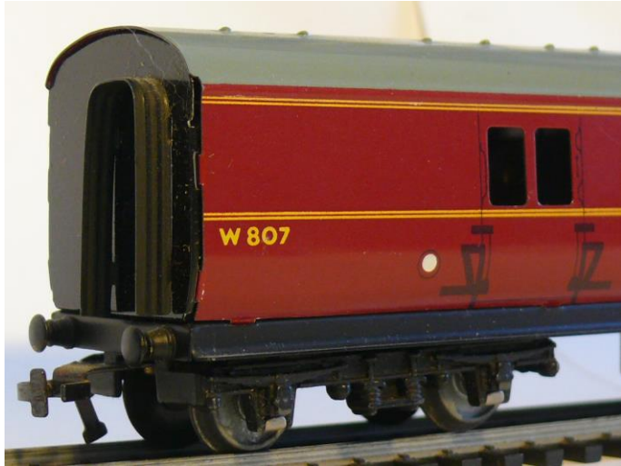
Note the prototypical correct asymmetric position of the corridor connection. This was to make sure that postal van corridors were only available between postal vans and the general public in a train could not enter a postal van.
