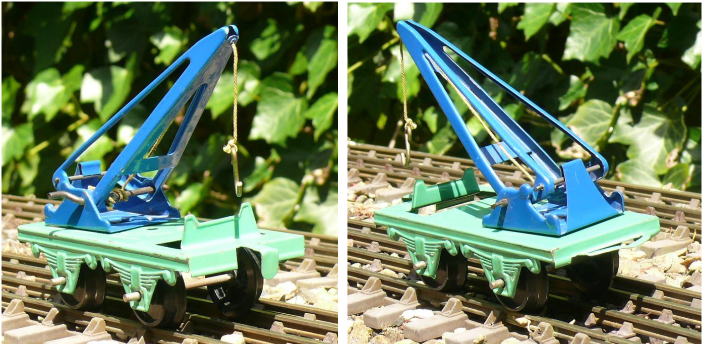
The crane body can be rotated and the jib can be lowered to rest on a support.
