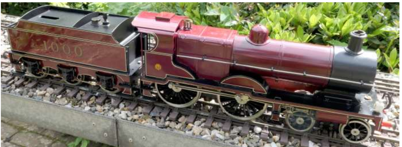
On the tender the spirit tank with filler and control can be seen; the oblong hole at the back is to be used for a handle for the tender feed water hand pump.
