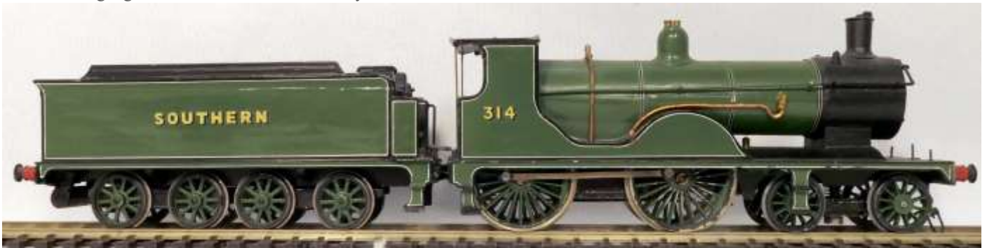
The next 00 gauge model of a Southern Railway T9 with a watercart tender is made from an unknown metal/brass kit.
