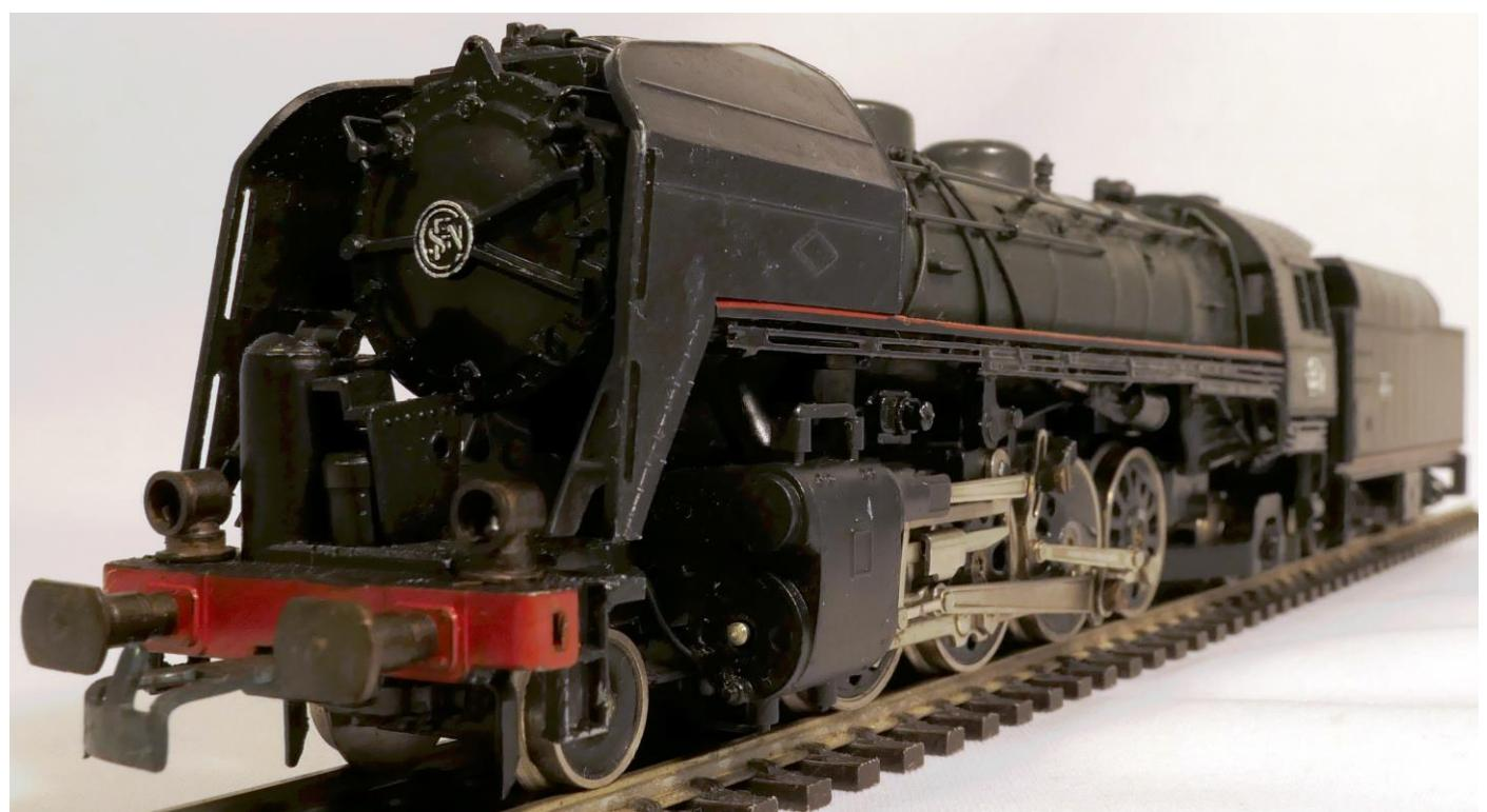
The SNCF 141TA are tender steam locomotives that were originally made for the Paris to Orléans Railway Company. They were built from 1911 to 1922 and were of a two-cylinder single-expansion type with Walschaerts distribution, with the driving rods on the second coupled axle (an unusual arrangement on 2-8-2's). Jouef announced models of 141TA416 in 1984. It is a nicely detailed plastic 2-rail DC model with a length of 15 cm.
