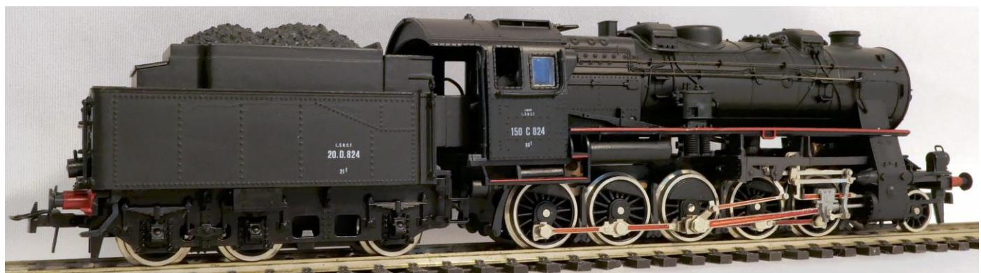
Here is a Jouef made model of the SNCF 150X in H0 gauge with catalogue number 8265 from the eighties. This 2-rail DC H0 gauge model has the motor in the tender. It has a plastic superstructure and is 26 cm long.
