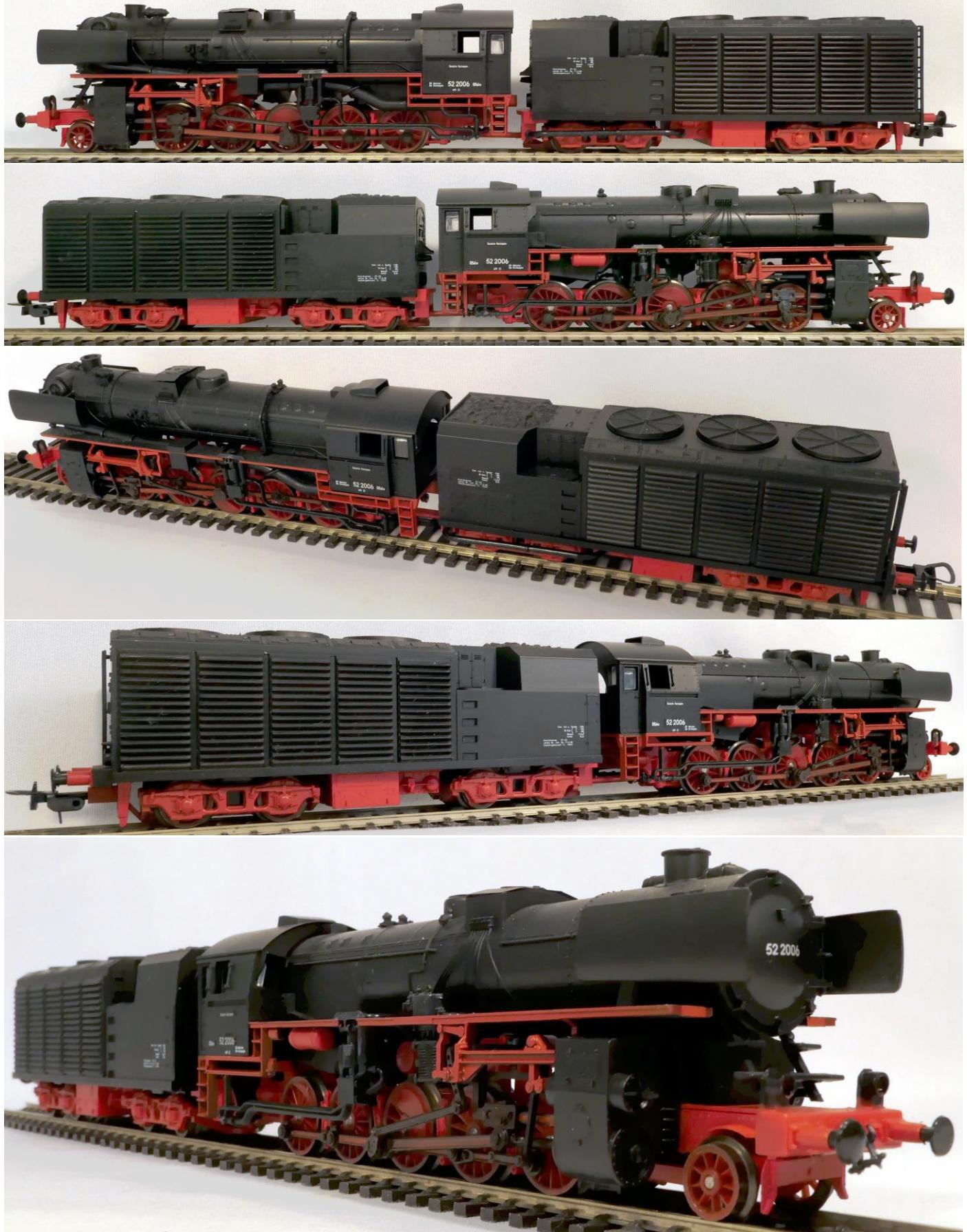
The locomotives of the Class 42.90 are steam locomotives of the Class 52 that were converted in 1951. They were equipped with a preheating boiler designed by Italian engineers Attilio Franco and Piero Crosti, (a so called Franco Crosti boiler). Märklin made with catalogue number 39160 a 26 cm long H0 gauge model of such a locomotive in grey photo colour. It is a metal and plastic 3-rail digitally controlled model.
