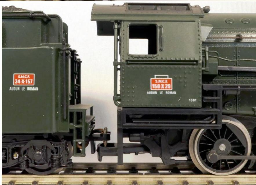
Märklin also made between 1965 and 1973 with catalogue number 3046, an SNCF 150X which was based on their 3-rail AC model of the German Class 44. It is a good running metal model with a length of 29 cm.
