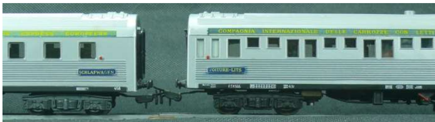
Right the coach with interior lighting, an electrical connection can be seen at the underside.
