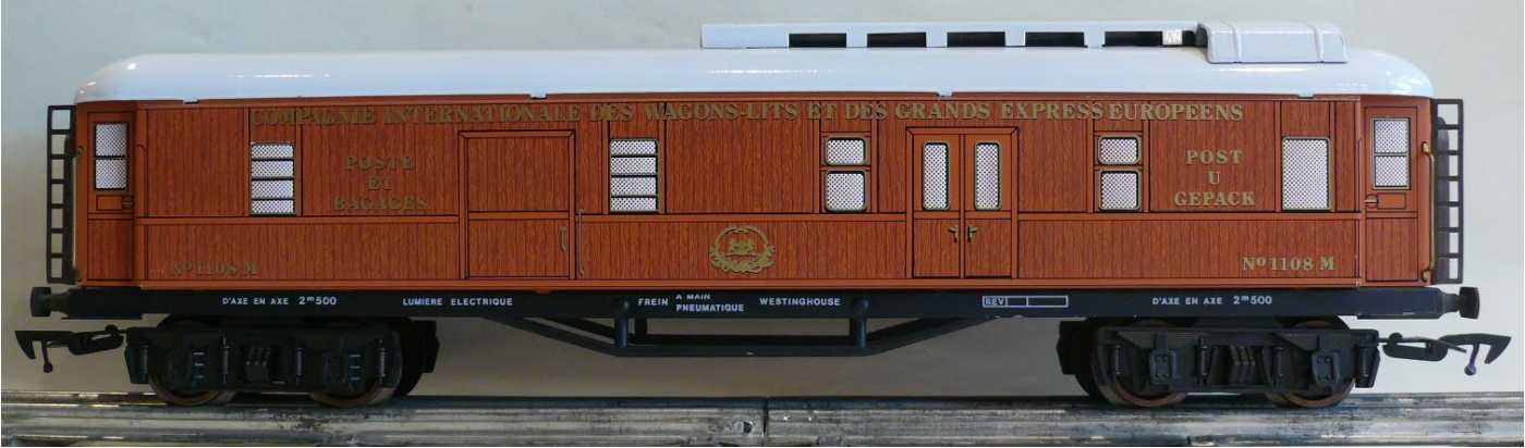
The postal compartment is at the right side and has a clerestory roof.
