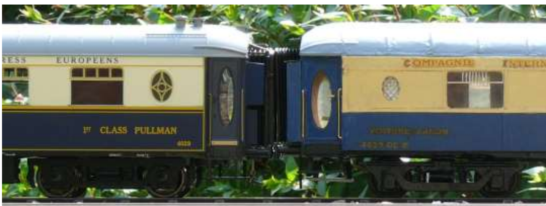
A comparison of Pullman cars; left an MTH plastic Flèche d'Or car and right this homemade wooden Côte d'Azur car.
