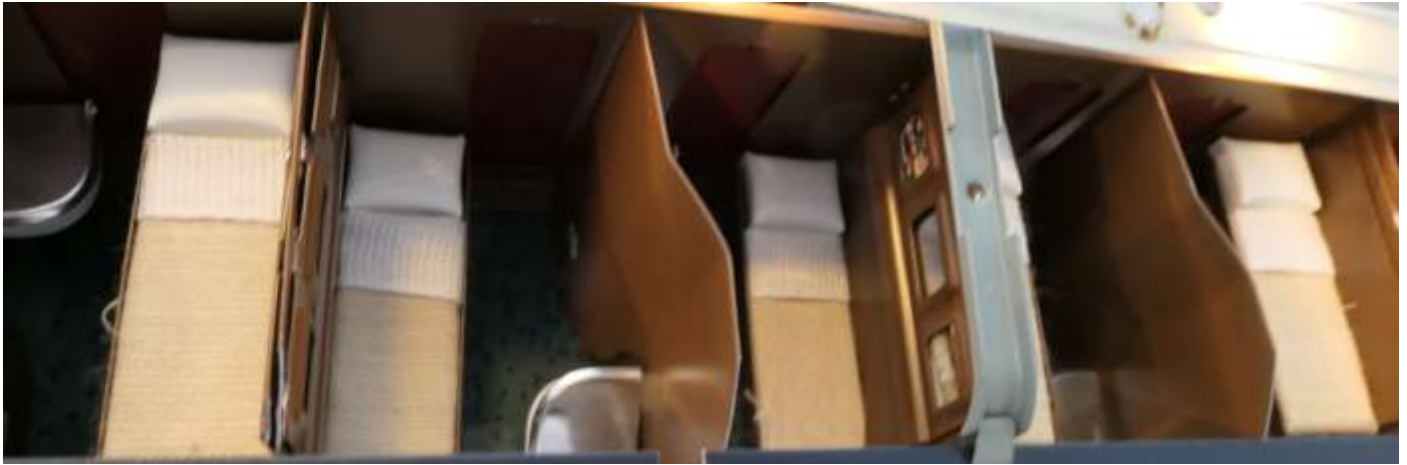
As mentioned this type sleeping car is named Z since it was the first with non-straight, i.e. Z like walls between the compartments to gain extra room for the wash basin, which is modelled correctly as can be seen in the picture above.
