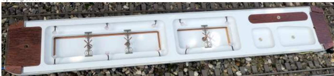
The roof is easily removed to show the detailed interior. The inside of the roof is also nicely detailed, including fans and lights
