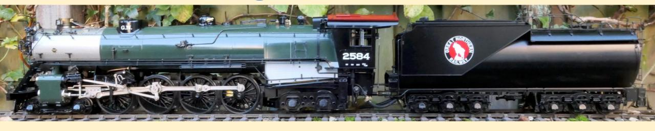
The 4-8-4 was a progression from the 4-8-2 and an example of the "Super Power" concept in steam locomotive design that made use of a larger firebox that could be supported by a four-wheel trailing truck, which allowed greater production of steam. The type was first used by the Northern Pacific Railway and called Northern, but some adopted different names.
