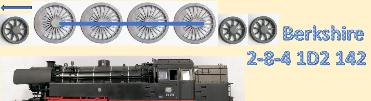
This locomotive type is most often referred to as a Berkshire. It resulted in the US from the requirement for a freight locomotive with even greater steam heating capacity. In Europe, this wheel arrangement was mostly seen in mainline passenger express locomotives and, in certain countries like Germany, in tank locomotives.
