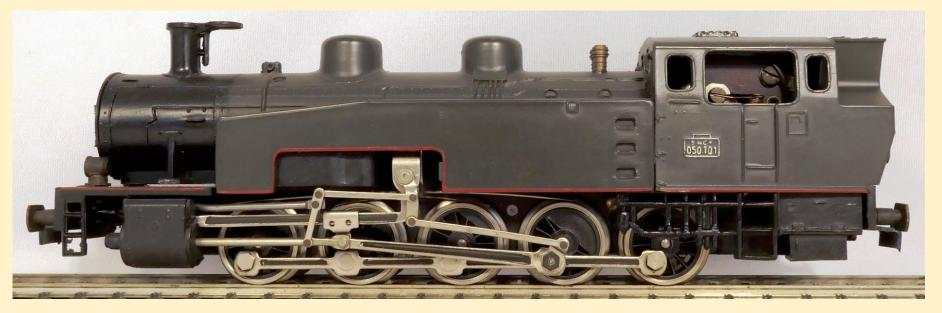
The lack of leading and trailing wheels makes this wheel arrangement unstable at speed, and it is a type usually confined to fairly low-speed work, such as switching, often as a tank engine version, transfer runs, slow-speed drag freight, or running over mountainous terrain.
