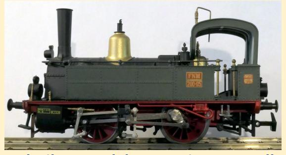
0-4-0 locomotives were built as tank locomotives as well as tender locomotives. The former were more common in Europe and the latter in the United States. The type, also called "Four Wheeler" was found to be so useful in many locations that they continued to be built for more than a century and existed until the end of the steam era.
