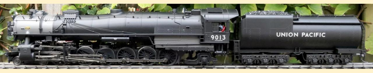
The Union Pacific 9000 class was the only class of steam locomotives with a this wheel arrangement ever to be built, also the 9000 class was the largest rigid frame locomotive ever built. These locomotives were used to increase the speed of freight trains in flat country, and were fairly successful.
