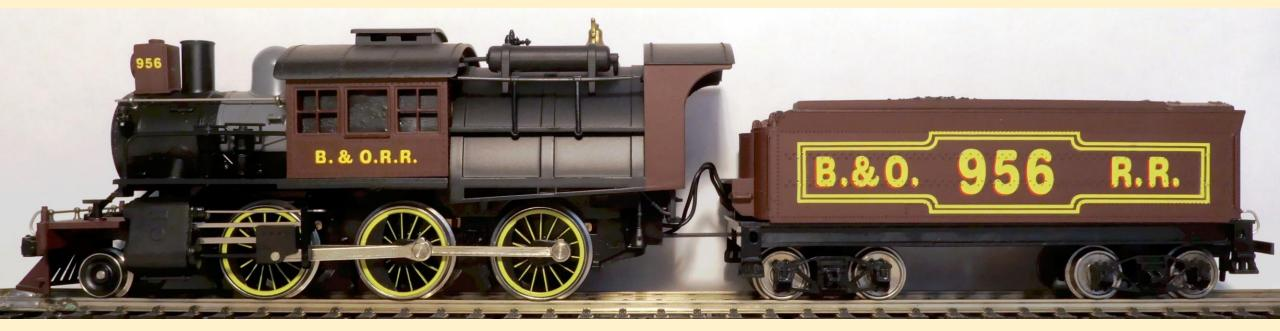
In the United States and Europe, the 2-6-0 wheel arrangement was principally used on tender locomotives. This type of locomotive was widely built in the United States from the early 1860s to the 1920s. In the United Kingdom, where locomotives are generally smaller than in the US, the 2-6-0 was found to be a good wheel arrangement for mixed-traffic locomotives.
