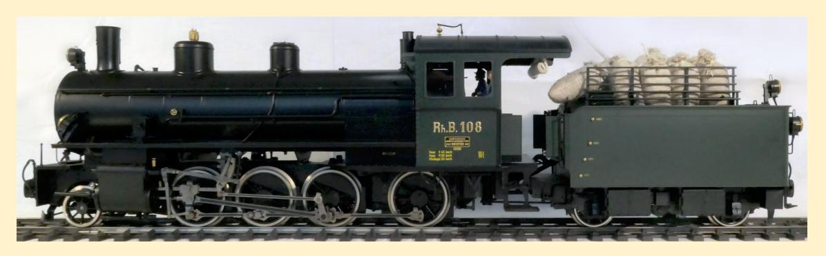
The Consolidation represented a notable advance in locomotive power. After 1875, it became very popular in the US and was built there in greater quantities than any other single wheel arrangement. Many larger narrow gauge engines around the world are Consolidations
