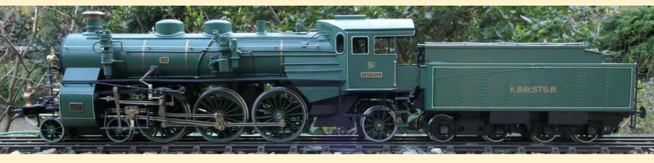
The 4-6-2 locomotive became almost globally known as a Pacific type after a locomotive built by the Baldwin Locomotive Works was shipped across the Pacific Ocean to New Zealand. On many railways worldwide, Pacific steam locomotives provided the motive power for express passenger trains.
