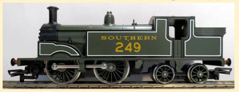
The 0-4-4 was only used for tank locomotives. In the UK 0-4-4T tanks were mainly used for suburban or rural passenger duties. In America, the wheel arrangement became known as the Forney, after a specific design of 0-4-4's, the Forney locomotive, became used on the narrow curves of elevated railways and other rapid transit lines.
