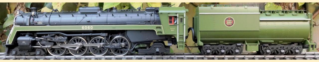
On the C&O RR it became necessary to doublehead "Pacifics" to get longer trains over the Allegheny Mountains. In 1910, the C&O turned to ALCO, they recommended a locomotive with eight drivers for traction to which they would add a four-wheel lead truck for riding stability. The result was a new wheel arrangement, the 4-8-2. It was named "Mountain" because it was developed to haul passenger trains over the Allegheny Mountains.
