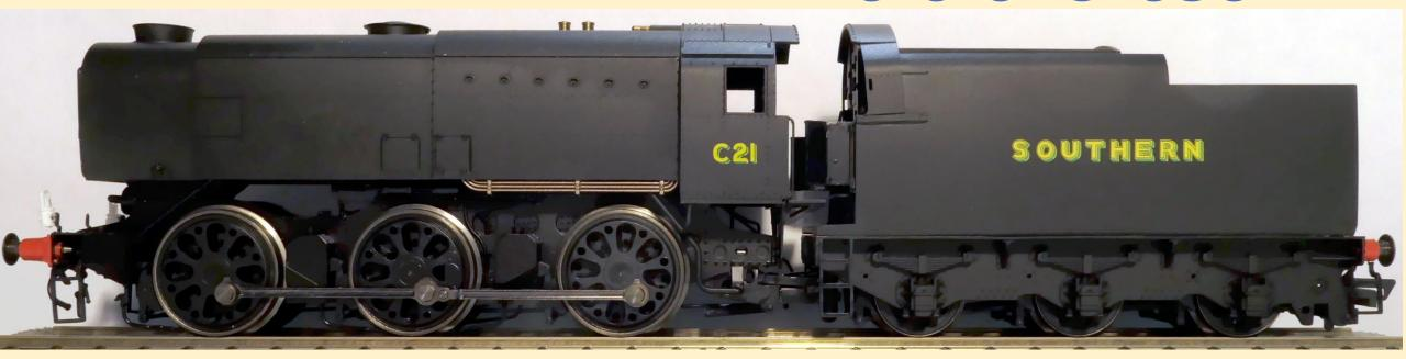
The 0-6-0 configuration was the most widely used wheel arrangement for both tender and tank steam locomotives. Locomotives of this type have all their weight pressing down on their driving wheels and consequently have a high tractive effort and factor of adhesion. They were also known as "Bourbonnais" and "Sixcoupler".
