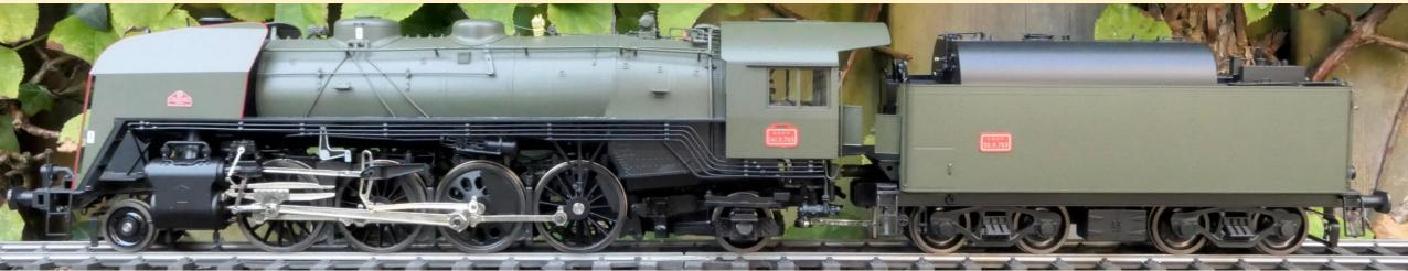
When introduced the 2-8-2 wheel arrangement allowed the locomotive's firebox to be placed behind instead of above the driving wheels, thereby allowing a larger firebox that could be both wide and deep. This supported a greater rate of combustion and thus a greater capacity for steam generation, allowing for more power at higher speeds. It was one of the more common configurations in the first half of the 20th century,
