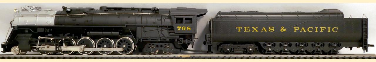
The 2-10-4 wheel arrangement originated and was principally used in the United States, but also Canada had this type and called it Selkirk. Some 2-10-4T tank locomotives also existed in eastern Europe.
