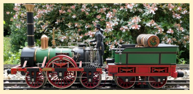
The 2-2-2 wheel arrangement is also known as "Jenny Lind" and was used on the first German steam locomotive Adler. The wheel arrangement both provided more stability and enabled a larger firebox than the earlier 0-2-2 and 2-2-0 types.
