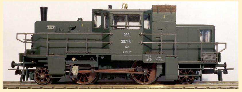
This wheel arrangement was widely used on passenger tank locomotives from 1870-1910. The vast majority of 2-4-2 locomotives were tank engines, i.e. 2-4-2T. The symmetrical wheel arrangement was well suited for a tank locomotive that is used to work in either direction. The type is named Columbia after a 2-4-2 locomotive showcased at the 1893 World's Columbian Exposition held at Chicago.
