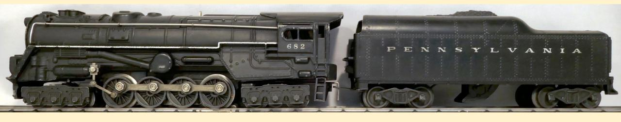
6-8-6 represents the arrangement of six unpowered leading wheels, eight powered and coupled driving wheels, and six unpowered trailing wheels. The only known example of the 6-8-6 wheel arrangement is the experimental Pennsylvania Railroad S2 steam turbine locomotive.
