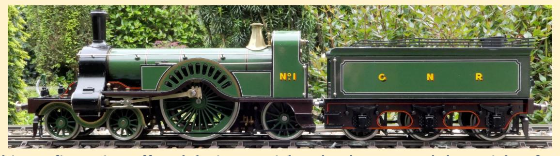
This configuration offered designers eight wheels to spread the weight of a larger locomotive, but prior to the invention of bogies created a long rigid wheelbase. The attraction of the 'single' was that, thanks to the large single driving wheels, a locomotive could obtain high speeds while the speed of the engine's pistons and valve gear remained relatively low.
