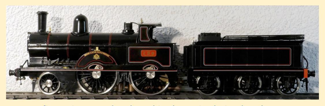
The 2-4-0 configuration was developed in the United Kingdom later as an enlargement of the 2-2-0 and 2-2-2 types, with the additional pair of coupled wheels giving better adhesion. Because of its popularity at that time with English railways it received the nickname of Old English.
