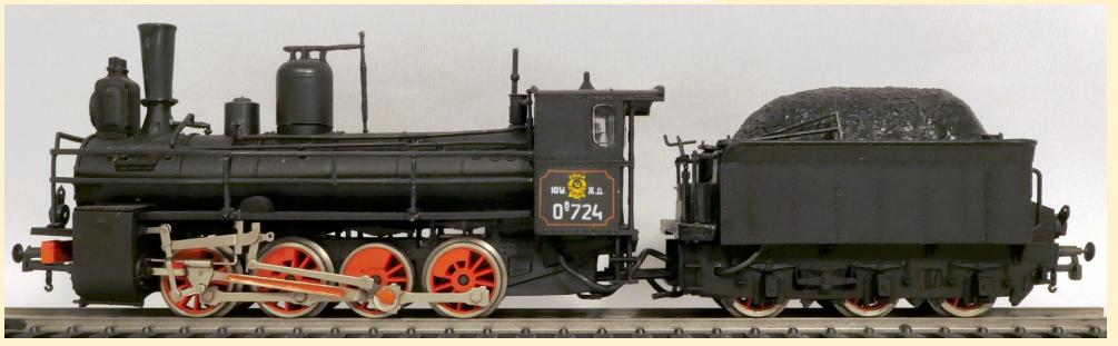
The wheel arrangement provided a powerful layout with all engine weight as adhesive weight, which maximised the tractive effort and factor of adhesion. This wheel arrangement appeared early in locomotive development in the US from the mid-1840s. It saw extensive use as a heavy switcher and freight engine in all countries including Russia.
