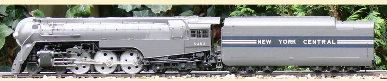
In France where the type was first used, it is known as the Baltic while it became known as the Hudson in most of North America. The type combined the basic design principles of the 4-6-2 type with an improved boiler and larger firebox increasing the steam-raising ability and giving more power at speed. The larger firebox necessitated additional support at the rear of the locomotive.
