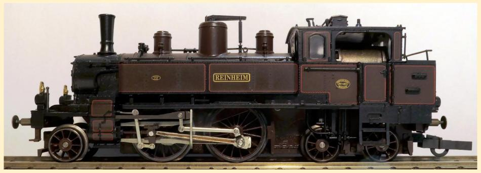
This configuration was only used for tank locomotives and did not have a "nick name". The unusual wheel arrangement does not appear to have been used on many mainline railways. It was however one of the configurations used on the Mason Bogie locomotives in the USA and on Bavarian tank locomotives.
