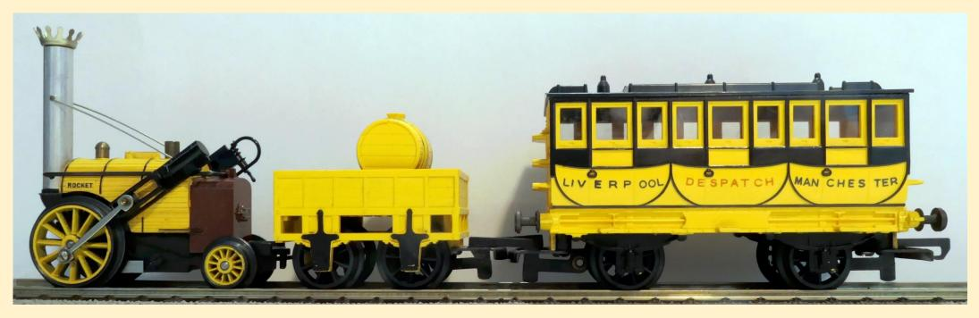
The 0-2-2 wheel arrangement is one that has two coupled driving wheels followed by two trailing wheels, with no leading wheels. The configuration was briefly built by Robert Stephenson and Company for the Liverpool and Manchester Railway amongs others for the famous Rocket locomotive.
