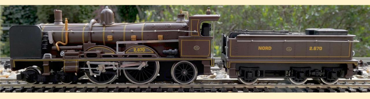
The 4-4-2 wheel arrangement is commonly known as the Atlantic type. One advantage of the type over its predecessor 4-4-0 was that the trailing wheels allowed a larger and deeper firebox to be placed behind the driving wheels. They had large-diameter driving wheels, adequate for higher speeds.
