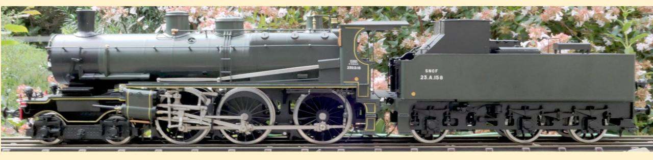
From the second half of the nineteenth century, the 4-6-0 was constructed in large numbers for passenger and mixed traffic service. A natural extension of the 4-4-0 wheel arrangement, the four-wheel leading bogie gave good stability at speed and allowed a longer boiler to be supported, while the lack of trailing wheels gave a high adhesive weight
