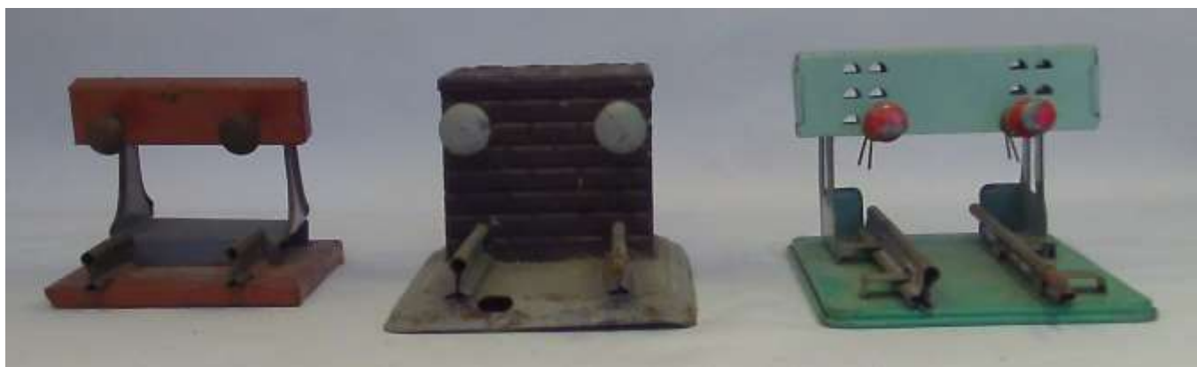
The next three are a bit messy; the left is marked Germany and looks as though it can bear no shock. The middle is a Bing buffer. The right is applicable for multiple gauges; also the buffer width and height can be adjusted on a rickety way.
