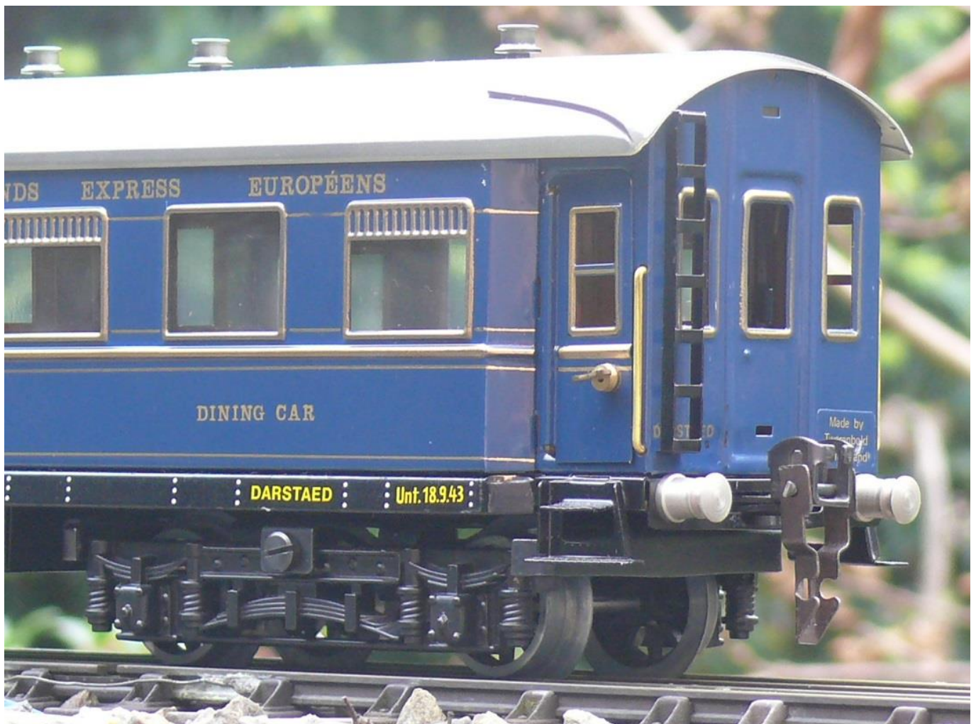
Märklin Fix coupler and very visible screw head on the bogie
