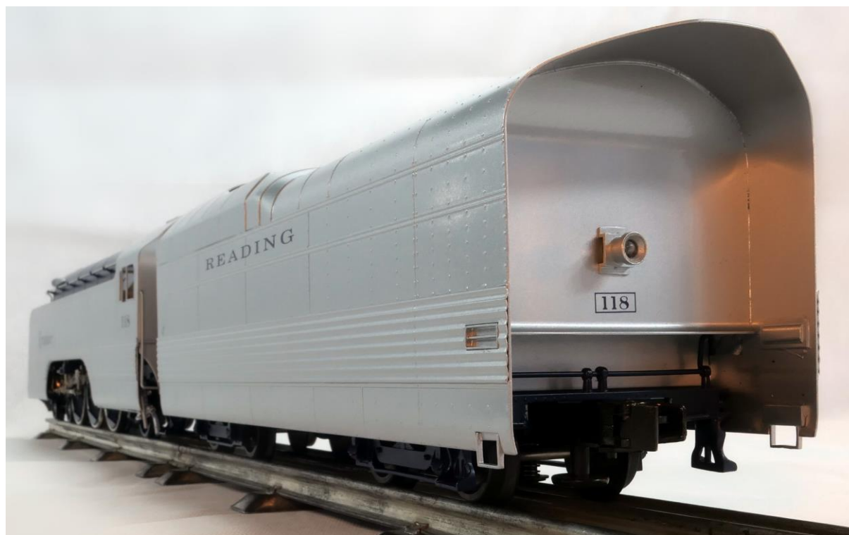
The tender has an overhang which wrapped around the first car.
