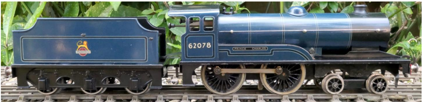
A post-war version of the Bassett-Lowke 0 gauge 4-4-0 “Duke of York” freelance locomotive (see 3.3.2.1) was named Prince Charles. Clockwork and electric versions were made. This locomotive is a clockwork version; it is 40 cm long.
